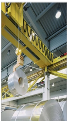
Crane Weighing System
